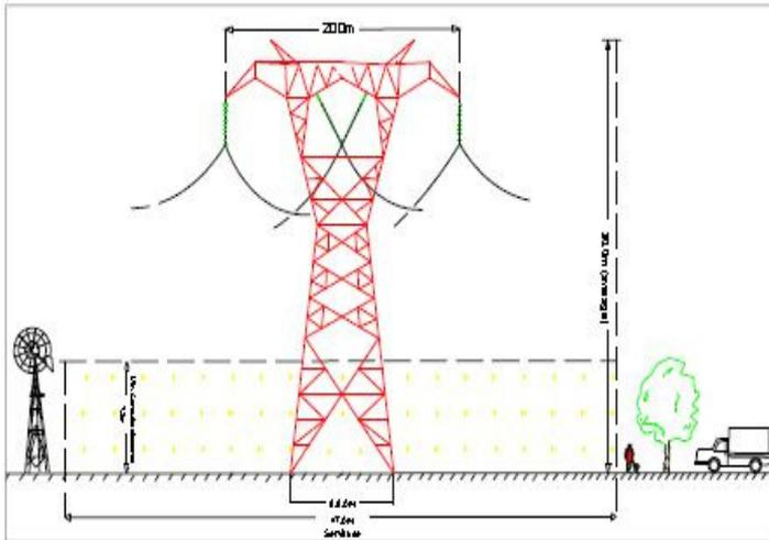
**Figure 5: Self-supporting Suspension Tower**
