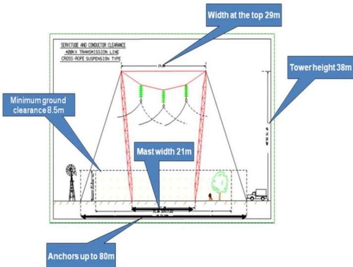
Figure 3: Cross Rope Suspension Tower
